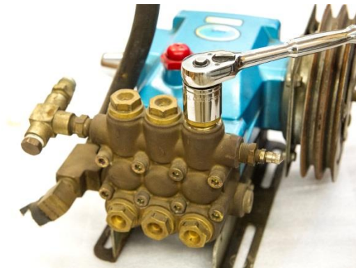
Figure 16: Removing valve plugs
