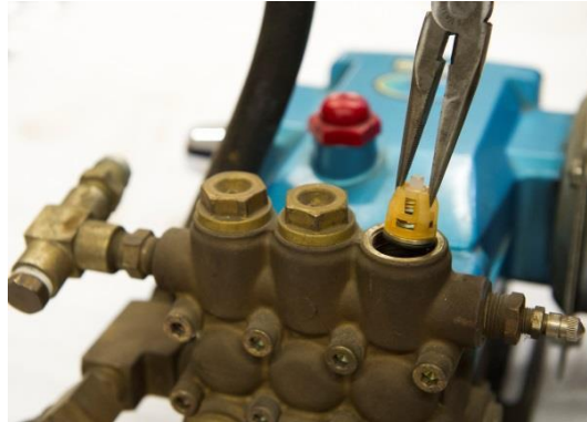
Figure 17: Removing the valve assemblies
