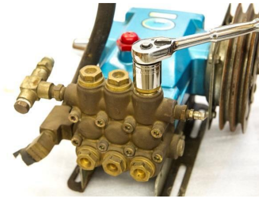
Figure 15: Removing valve plugs
