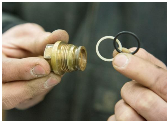
Figure 14: Examining the O-ring gaskets
