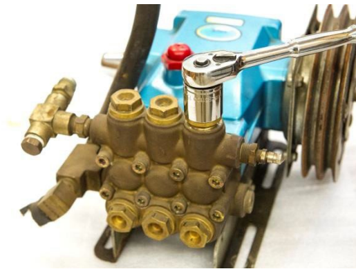
Figure 13: Removing valve plugs
