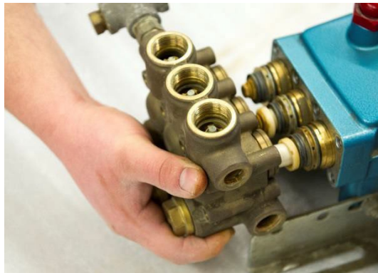
Figure 17: Removing the manifold head
