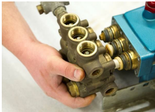
Figure 20: Removing the manifold head
