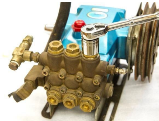
Figure 16: Removing valve plugs
