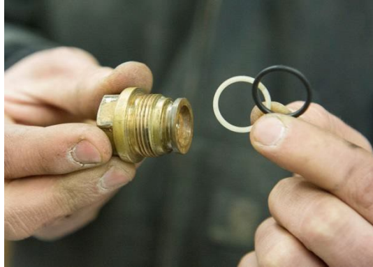
Figure 17: Examining the O-ring gaskets
