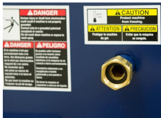
Figure 6: Water connection in the back of the machine
