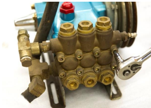
Figure 19: Removing the cap bolts
