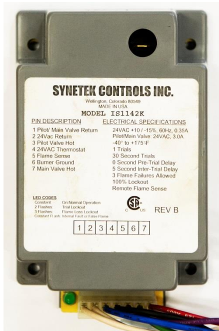
Figure 25: Intermittent ignition device front with chart of fail codes.
