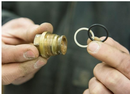
Figure 17: Examining the O-ring gaskets
