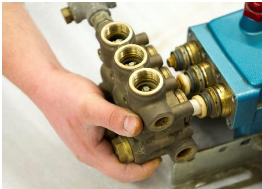
Figure 20: Removing the manifold head
