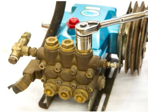
Figure 16: Removing valve plugs
